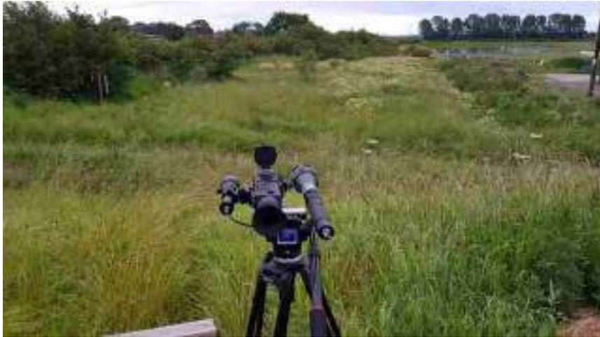
Fig. 8-1 Laserfence handheld mounted on a tripod, and overlooking fields at RSPB. Also mounted was a night vision scope and IR illuminator
